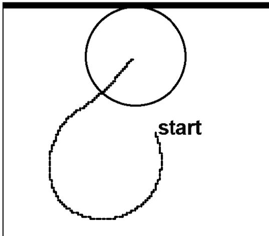
**Figure 0-3** An example of low-fitness behaviour typical of a robot in the first generation. It makes a continuous line up to the point that it crashes into the arena wall. The robot does not change its pen state during the whole trial.
