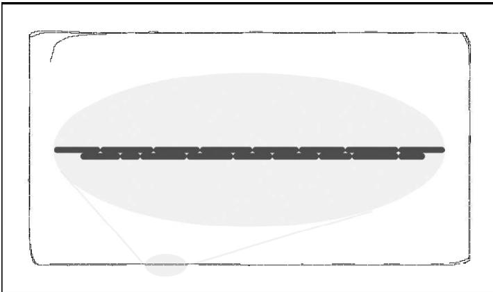
**Figure 0-5** Performance of a high fitness individual after 500 generations. The robot completes one circuit of the arena with its pen down by following the walls. On its second circuit it sweeps left and right over the line, marking line segments parallel to the line it had previously left.
